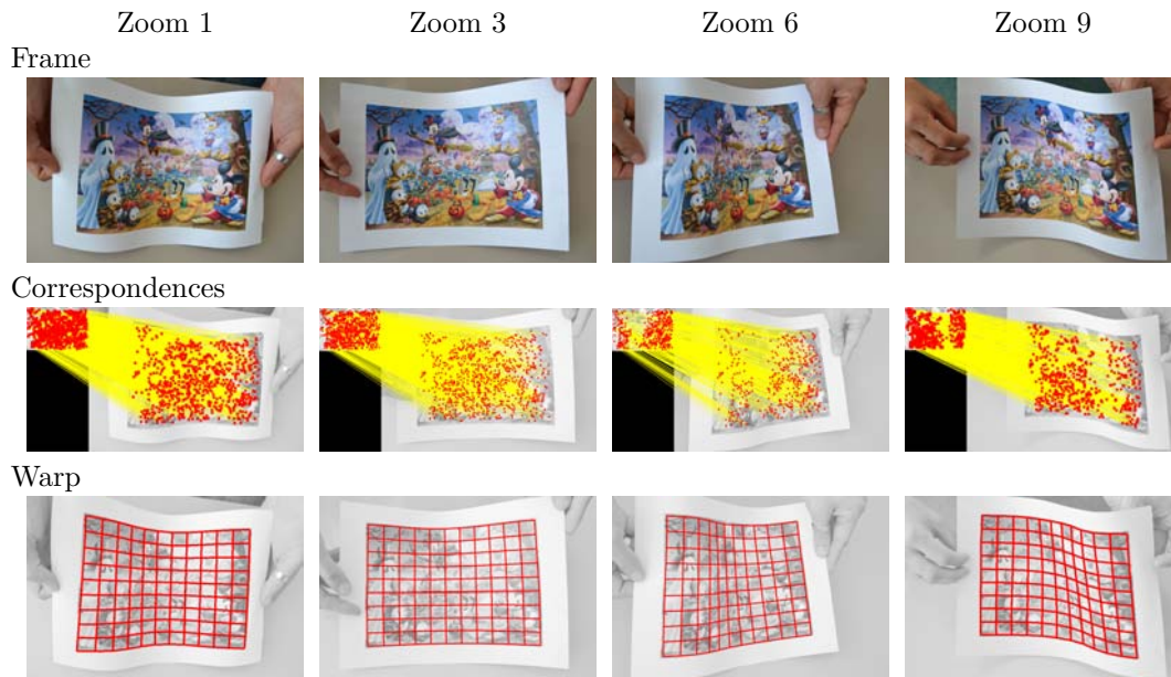
Figure 18: The zooming paper dataset. Sample frames, point correspondences and estimated image warps.
